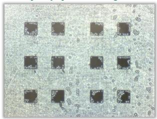
Apertures are clogged and solder paste is smeared out on the stencil.
