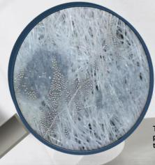
The 3D structure embeds the solder paste particles in the fabric and safely transports them away from the stencil.
