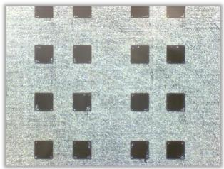
Apertures are clean and there is no smearing of solder paste on the stencil.
