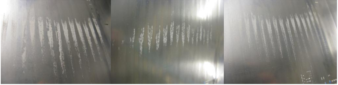
Figure 20 – Remaining solder paste after the first cleaning cycle, A (left), B (middle) and C (right).
