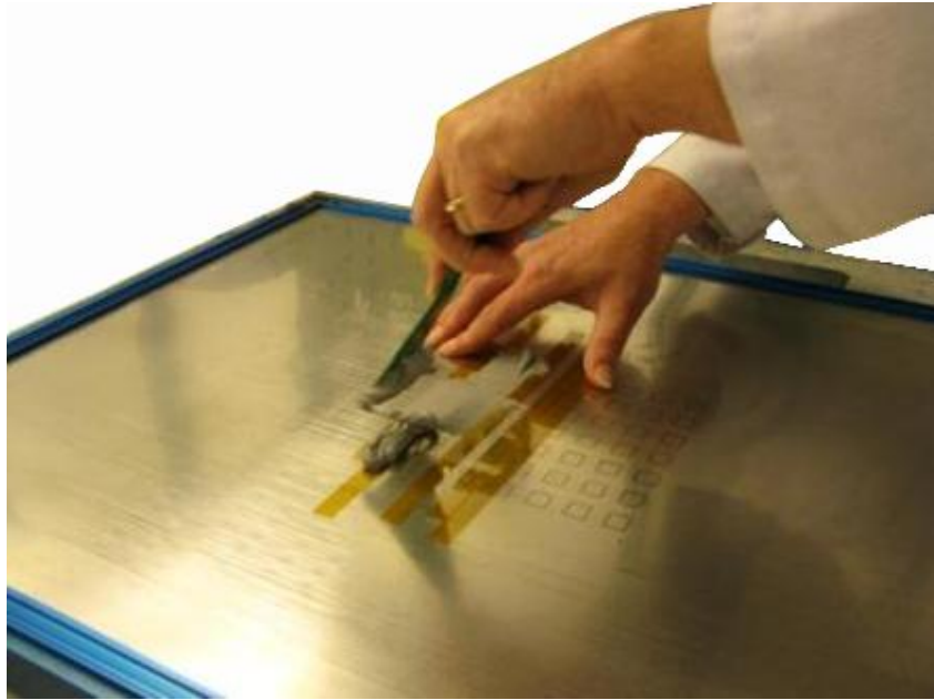
Figure 18 – Manual screenprinting of solder paste on bottom side of stencil
