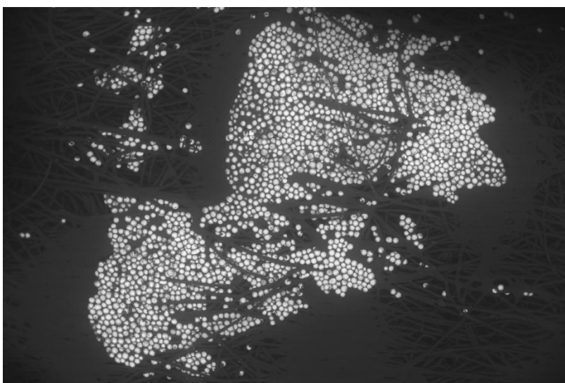
Figure 23 – Cleaning paper B, entrapped solder particles.
