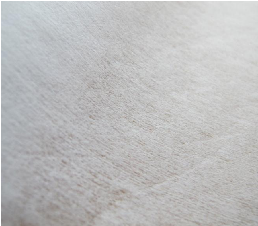
Figure 7 – Photo of cleaning paper C. Even surface, darker “lines” with less material.
