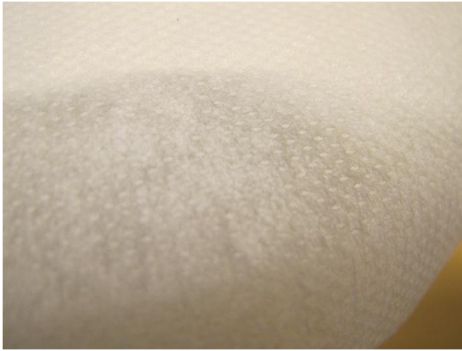
Figure 6 – Photo of cleaning paper B. Wave formed surface because of regular imprints.
