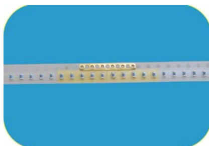
Demonstration: Downside of the connecting reel.
