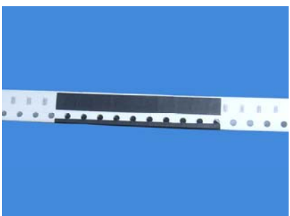
Step 6: Downside of connected carrier tape.
