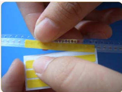
Step 7: Peel off the paper liner
