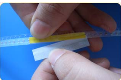
Step 7: Peel off the paper liner.
