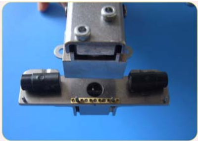
Step 1: Put Splice Clip into splice tool.
