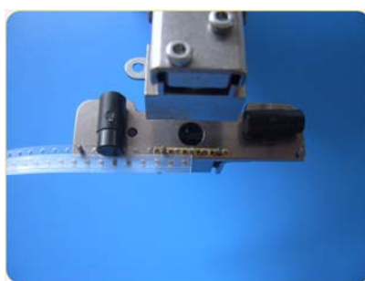
Step 2: Put one pre-cut reel into splice tool.
