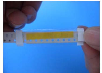
Step 6. Press the splice tape with hole in the connecting reel tightly.
