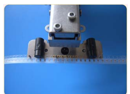
Step 3: Put another pre-cut reel into splice tool.
