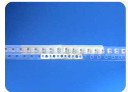
Demo.: Downside of connected tape.
