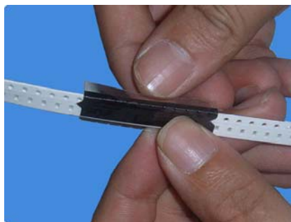
Step 4: fold down the splice tape.
