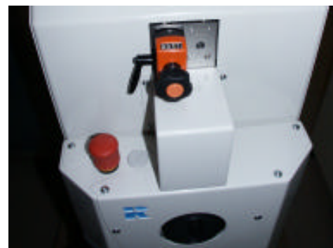
Adjustment regarding PCB thickness and overlap, emergency stop switch and hand crank for conveyor width adjustment
