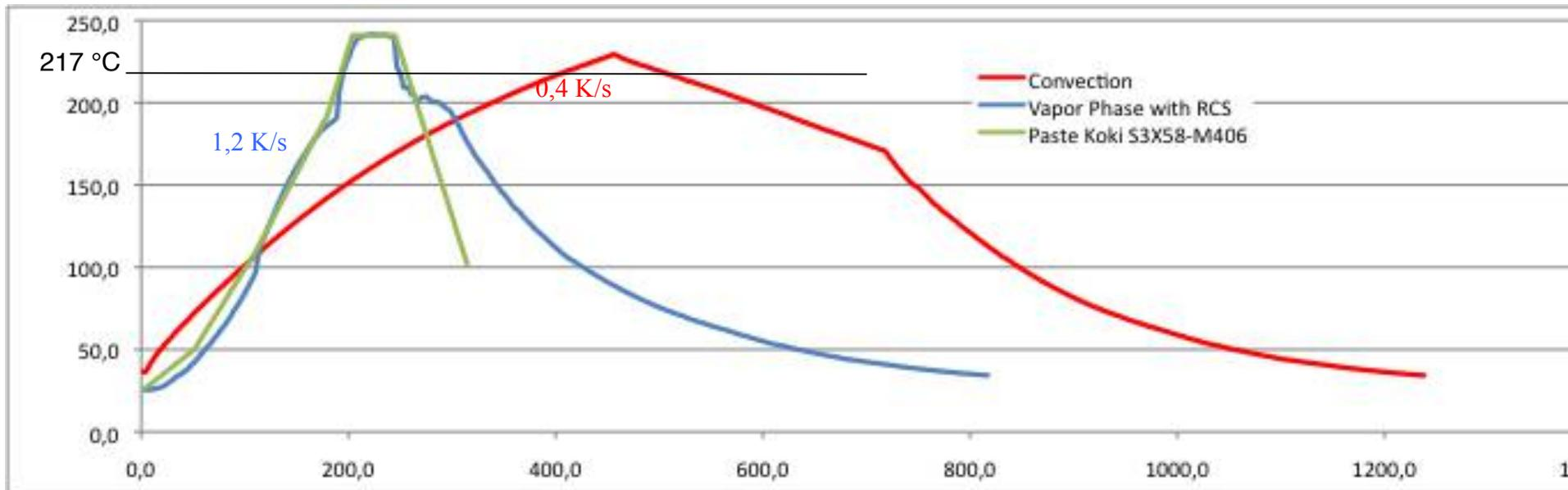
Solder profile of a ceramic unit (0,4 K/s vs 1,2 K/s) in direct comparison of Vapor Phase and Convection
